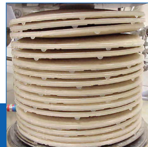
Cell deformities after heat treatment
