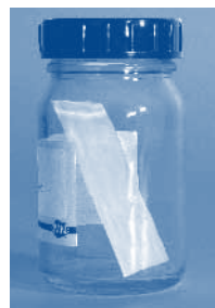
Fig. 2: TLC sheet in the developing chamber
