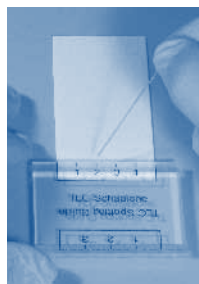
Fig. 1: Applying of samples on to a TLC sheet with capillary and spotting guide
