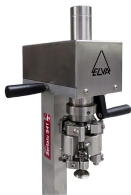
A close-up view of the manual capping machine, showing the capping head and the base. The ELVA logo is visible on the side of the machine.
